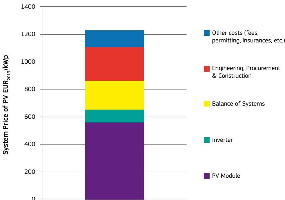
Fig. 12: Price breakdown of utility-scale PV system
